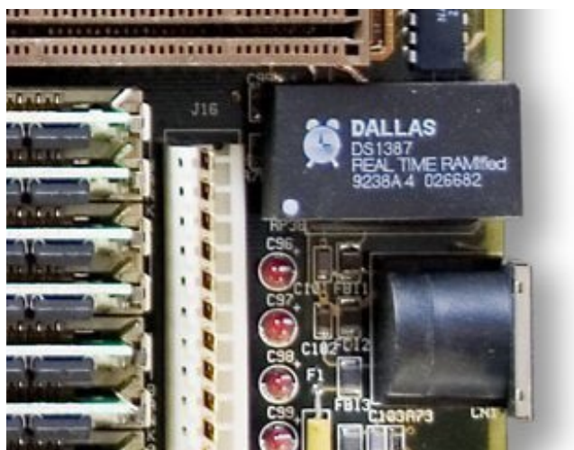
This image shows a computer motherboard with a Real Time Clock called the
