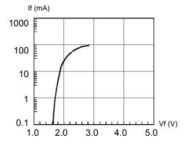
Fig. 3 Forward Current vs. Forward Voltage
