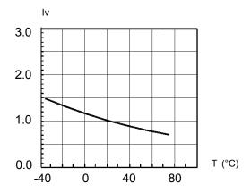
Fig. 6 Relative Luminous Intensity vs. Temperature
