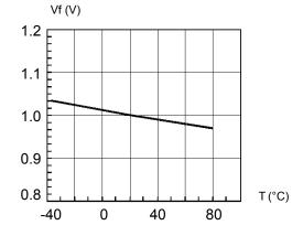
Fig. 5 Forward Voltage vs. Temperature
