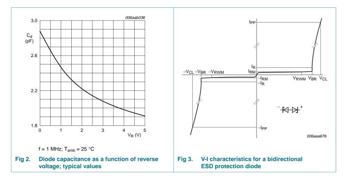
Ultra low capacitance bidirectional quadruple ESD protection arrays
