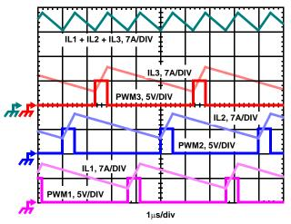
FIGURE 2. PWM AND INDUCTOR-CURRENT WAVEFORMS FOR 3-PHASE CONVERTER
