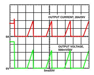
FIGURE 6. OVERCURRENT BEHAVIOR IN HICCUP MODE
