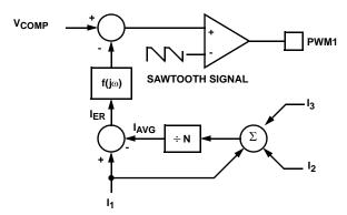
FIGURE 5. CHANNEL-1 PWM FUNCTION AND CURRENT-BALANCE ADJUSTMENT
