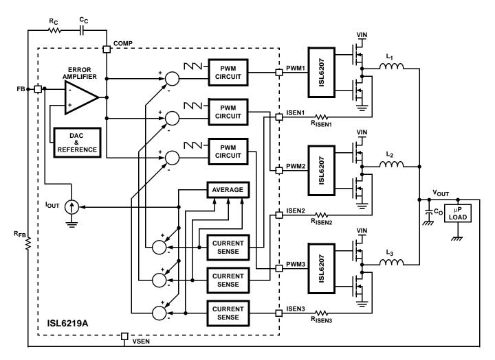
FIGURE 1. SIMPLIFIED BLOCK DIAGRAM OF THE ISL6219A
