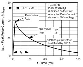
Fig. 3 - Pulse Waveform
