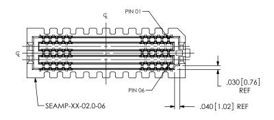
FIG. 4 -10: 10 ROW (SAME AS FIG. 1, EXCEPT AS SHOWN) (SEAMP-30-02.0-X-10-XX SHOWN) (SOME CENTER FEATURES NOT SHOWN FOR CLARITY)
