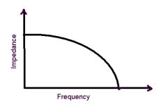
Figure 7– Ideal capacitor frequency response
