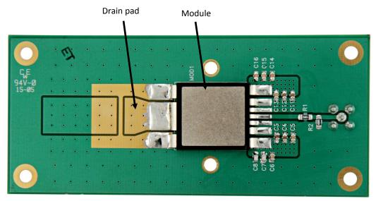
Figure 2 Bottom side of development board
