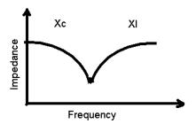
Figure 8- Capacitor frequency response due to self inductance
