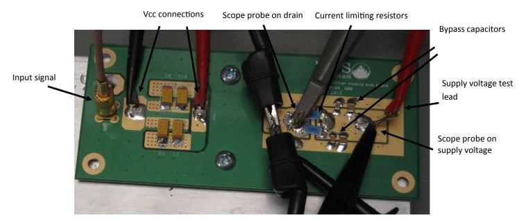
Figure 12 Board connections
