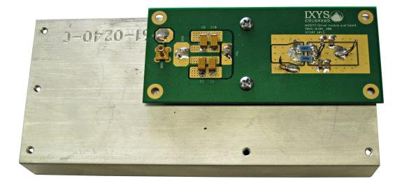
Figure 4 Board mounted to heatsink\*\*
