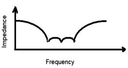
Figure 10- Broadband impedance lowered
