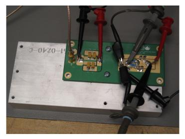
Figure 11 Demonstration board mounted to heat-sink
