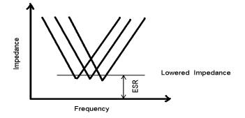
Figure 9- Over-lapping impedance curves
