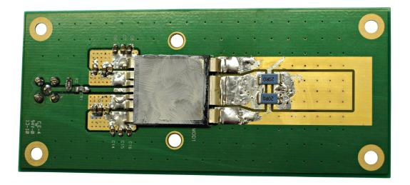
Figure 3 Application of thermal grease
