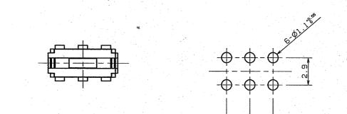
7.5 Reference dimension drawing of mounting hole 取付元推奨寸法図 (Tolerance 公差: ±0.05) (t=0.8mm)
