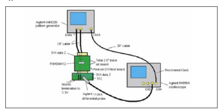
Figure 1. TMDS TP2 Tx eye compliance test setup
