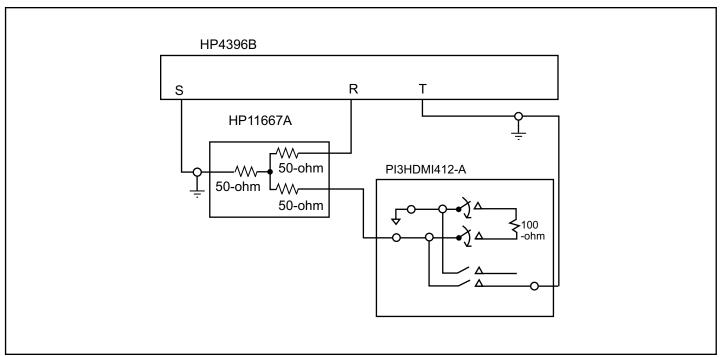
Fig 2. Off-isolation setup
