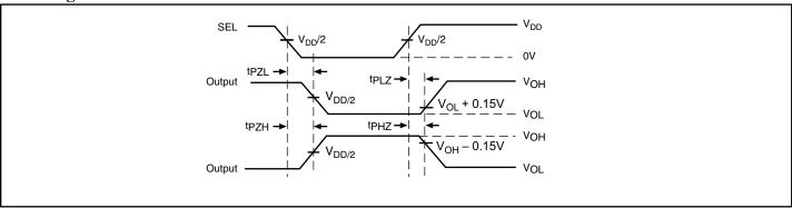
Voltage Waveforms Enable and Disable Times
